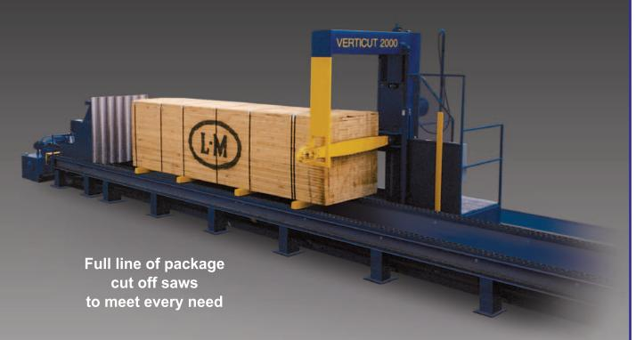
The saw allows a single operator to complete a quality cycle under 55 seconds, Our shorter, stiffer bar is guided vertically through the lumber package, allowing it to consistently maintain cutting tolerances of  $\pm$  0.040". This specially designed, precision chain saw's thin 3/8" kerf gives you more efficient lumber recovery and a surface finish as good or better than a conventional trim saw.
