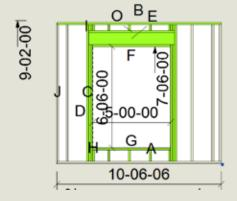
Here is a fairly typical 2x6 exterior wall. Following the specified nailing schedule this wall would have 237 nails for the framing portion of the wall. 96 of these (40%) would be installed by one operator using the Terminailer.
