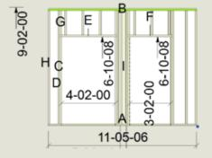
The 2x4 interior wall panel, the nailing schedule specifies 153 total framing nails with 81 driven automatically by the Terminailer for a total of 52%.
